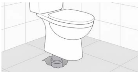
ANTES - SIN MANGUITO ACORTABLE BEFORE - WITHOUT ADJUSTABLE PAN CONNECTOR
